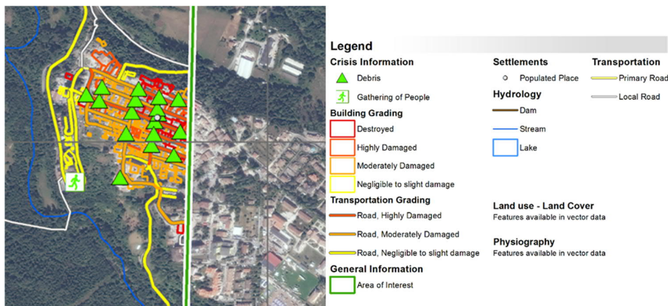
Figure 60: Extract of Layer Showing Part of Damaged Buildings and Roads during Amatrice Earthquake in August 2016 with Legend to the Right Source: Copernicus Emergency Management Service (© 2019 European Union), [EMSR177]
